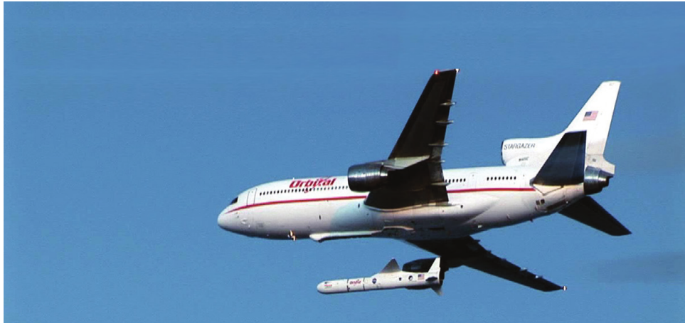
Figure 3.1: A Pegasus XL Launcher being Air-launched by the Stargazer Aircraft at the moment of release [30].
