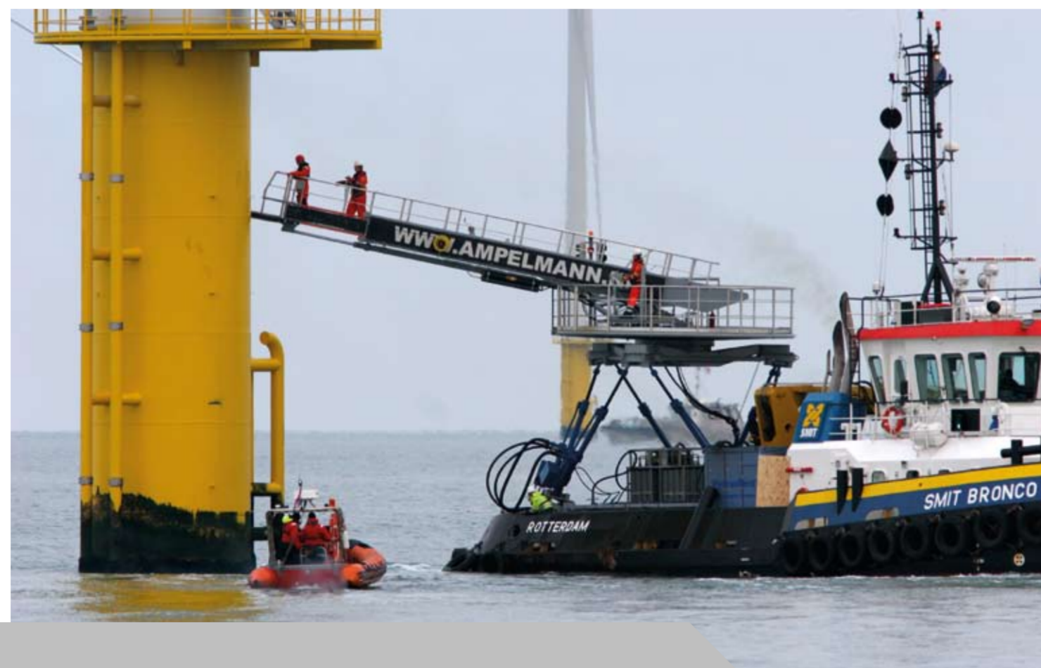
Delft University access system 'Amplemann' was positioned on board the 'Smit Bronco' for its first operational trials.
