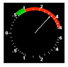
The Instantaneous Vertical Speed Indicator (IVSI) (Figure 5 above) shows the aircraft is climbing at 3,300ft/min, the range of forbidden vertical speed is 1,000 to 6,000ft/min and recommended vertical speed is between 600 and 1,000ft/min.
