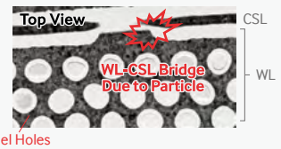
Figure 12. The major structural failures that can occur in NAND flash memory
