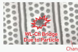
Figure 12. The major structural failures that can occur in NAND flash memory
