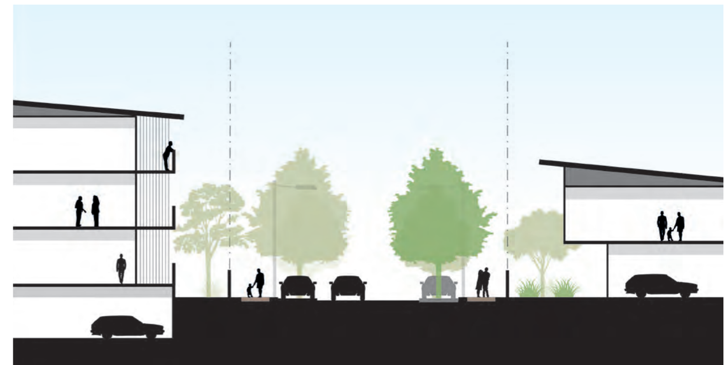
Indicative street cross section – Typical Local Street
