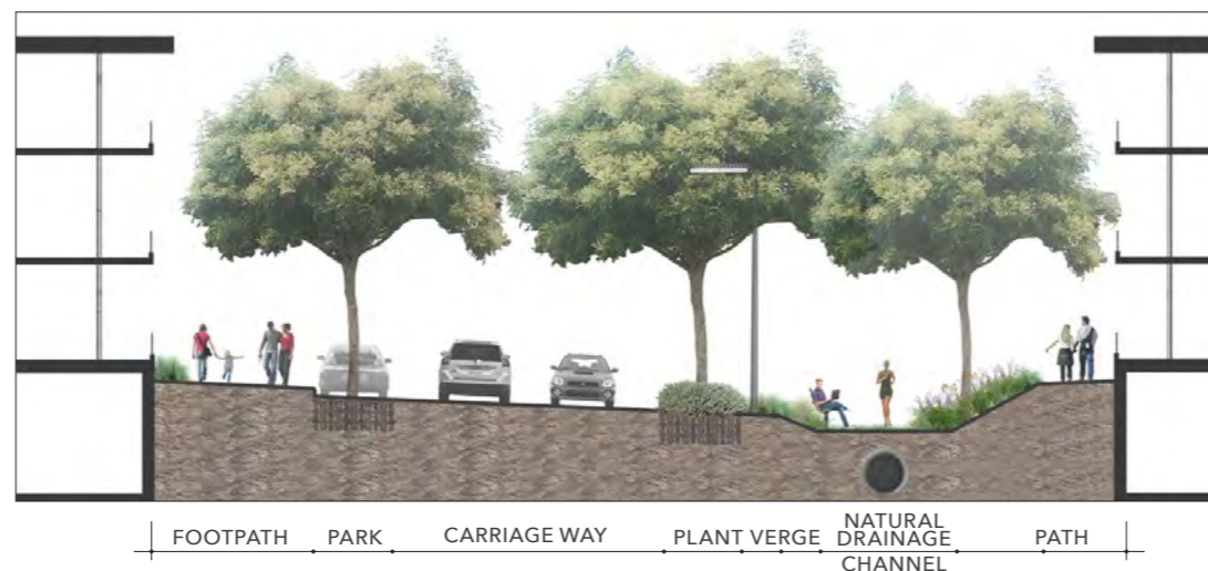
Indicative cross section – North-South Avenue (A)
