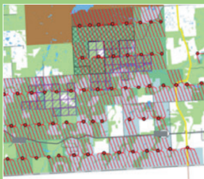
Well pad placement and HDD visualization: maximal resource access with no constraints
