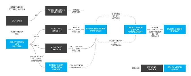
Dolby Vision is compatible with a wide range of video codecs. It's currently qualified with HEVC and AVC decoders. An implementation will take the source stream (typically a video elementary stream with interleaved base-layer access units [AUs], enhancement-layer AUs, and metadata reference processing units [RPUs]), split it, and feed the encoded streams through decoders.
