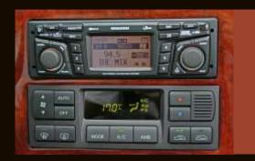
**Multimedia System and Automatic Climate Control.** GPS navigation system, Hi power amplifier, 5 speaker and 6 disc CD changer under the bonnet (optional).
