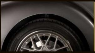
Wheels. 17"  $\times$  7" two piece magnesium alloy rims c/W polished stainless steel edge rim with Kevlar enforced Continental tyres 225/45 R17 91W.
