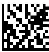
In the past 20 years, 2D Data Matrix codes have become an integral part of tracking and traceability in manufacturing and production facilities around the world, from direct part marks (DPM) on automotive parts and PCBs to printed codes on pharmaceutical products, where small size and readability are vital.
