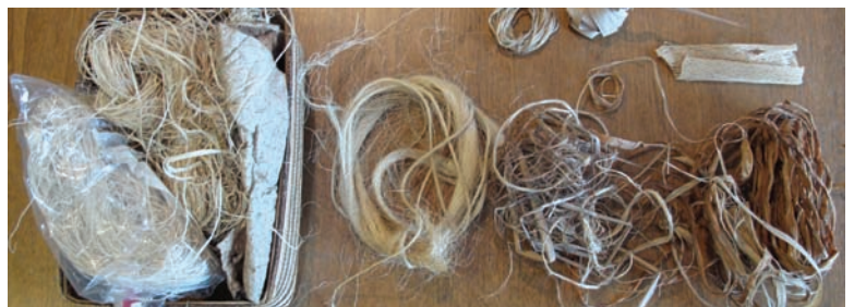
Samples of Amazon fibers. From left to right: Moriche palm fiber, wasp nest (in basket), shiki, tavarí of different qualities. Above: blond tavarí, palm and inner bark.
