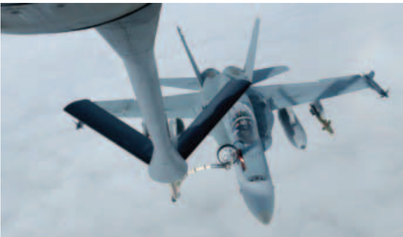
A RAAF F-18 aircraft refuels from a USAF KC-135 during a combat mission over Iraq © Defence Dept.
