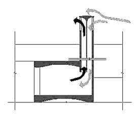
Figure 1: traction and suction in wind-catcher.
