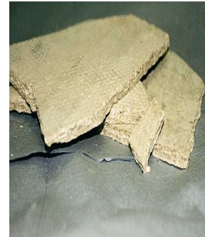
Flat asbestos cement sheeting
