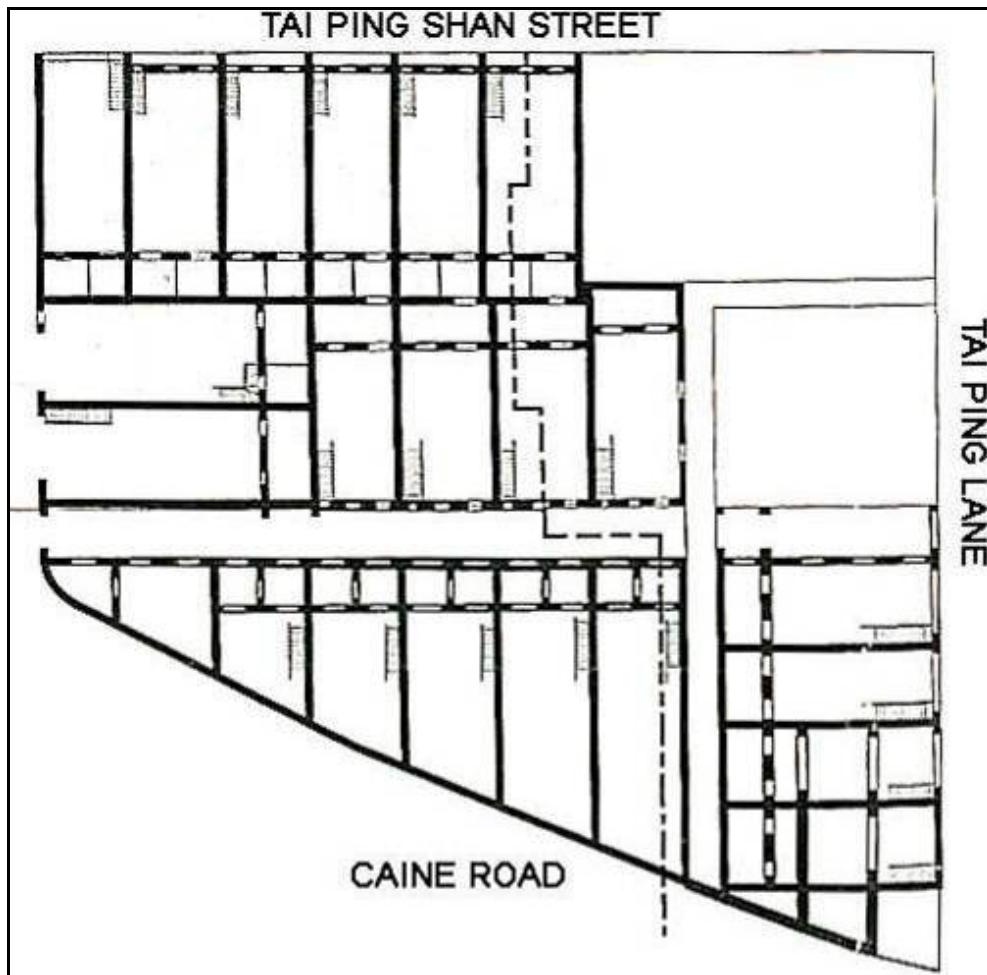
Fig. 8 Block plan of several rows of early Tong Lau at Tai Ping Shan, early 1880s. (Source: Chadwick's Report (1882) in Faure 1997: 44)
