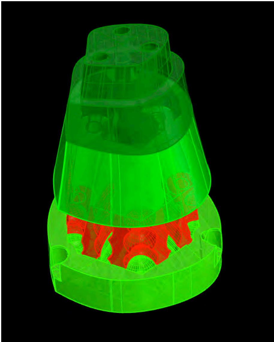
Figure 114 - cutaway view of the base of Prototype Column showing subtractive ellipsoid internal geometry
