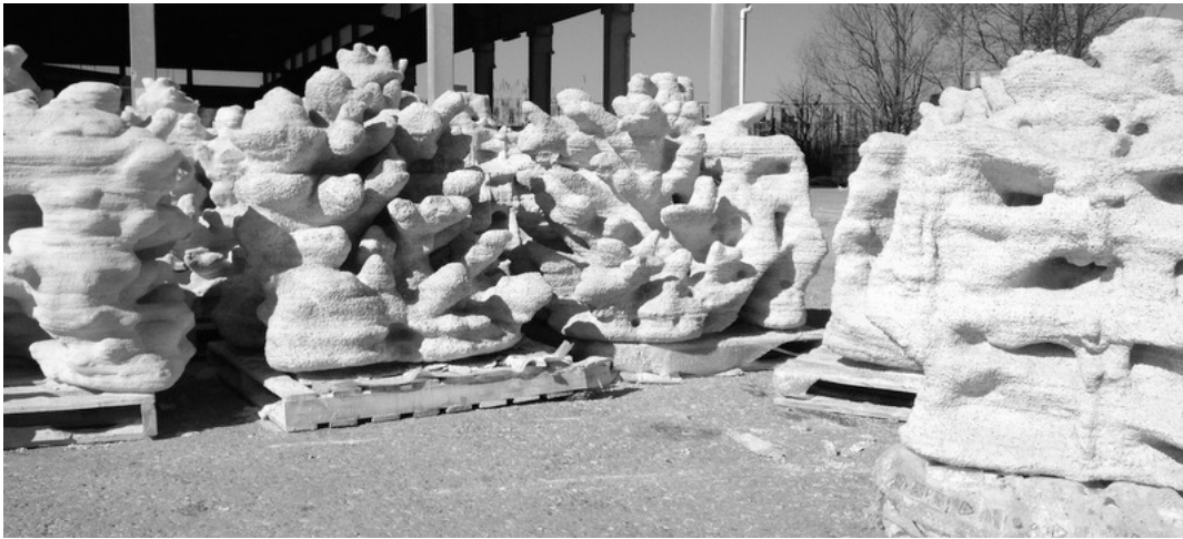
Figure 194 - Eight printed reef modules at the D-Shape factory in Tuscany. Commissioned by Sustainable Oceans International. Designed by James Gardiner
