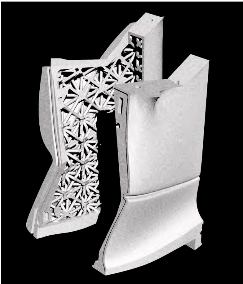
Figure 141 - Split panel showing internal geometry, rebates for plate stirrups & lifting and dowel slots
