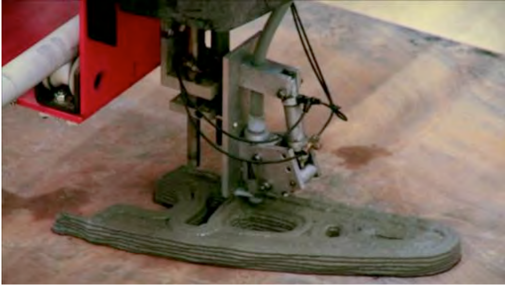
Figure 17 - Concrete Printing nozzle. Image source - http://www.rationaloptimist.com/blog/print-your-own-organs - Accessed on the 9th August 2011
