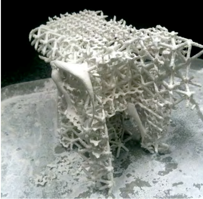
Figure 185 - One of the printed blocks after having the unbonded powder removed. Photo by James Gardiner
