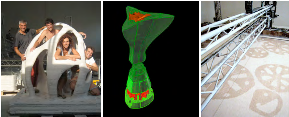
Figure 4 - (a) Embedded with D-Shape team (b) Prototype column design (c) Prototype column being printed in sections
