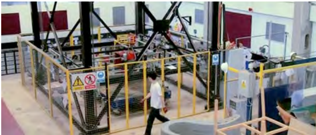
Figure 16 - Concrete Printing Machine. Image courtesy of Dr Richard Buswell
