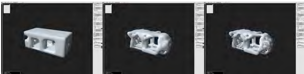
Figure 60 - Topostruct TM optimisation test for Villa Roccia 2009
