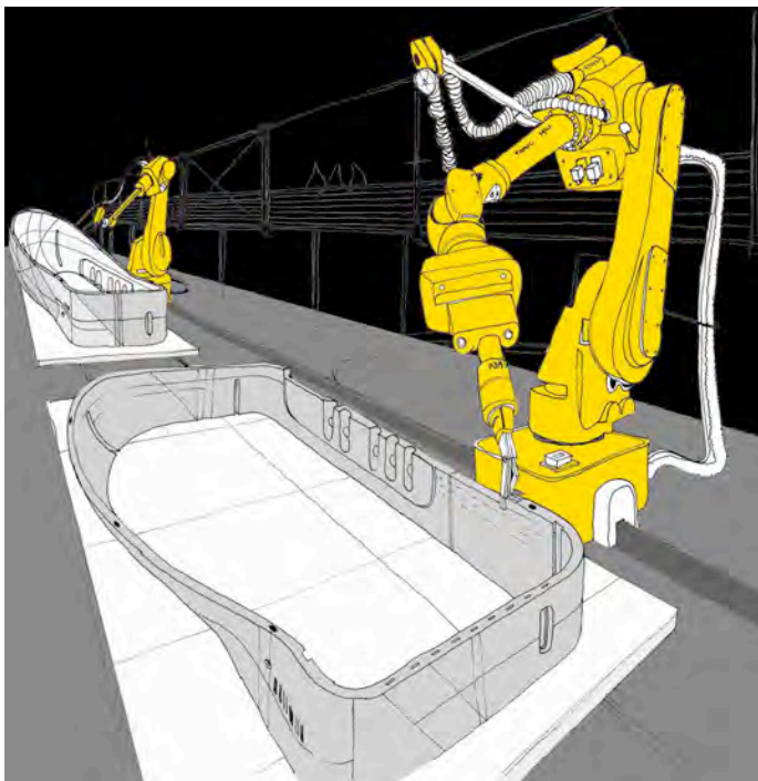
Figure 83 – Freefab shell production using a modified Contour Crafting system on a production line. James Gardiner UTS 2004
