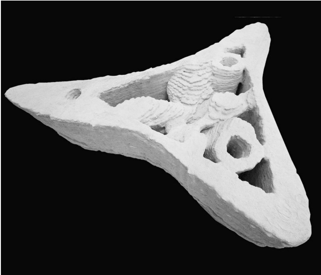
Figure 138 - One of the Roccia Prototype column sections as printed. Note the internal stepping where the curve is not in the direction being printed. Photo James Gardiner
