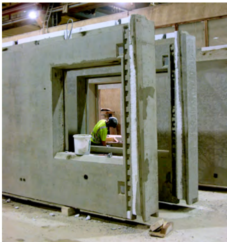
Figure 69 - Skanska Precast concrete panel factory in Stragnas, Sweden. Composite panels of timber and plasterboard being lifted into place on site in Stockholm, Sweden. Photos by James Gardiner
