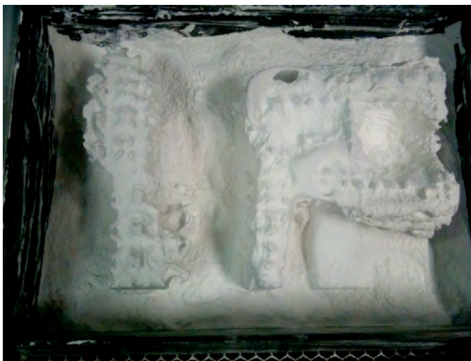
Figure 184 - Two blocks being removed from the Z-Corp 3D printer at RMIT. Photo by James Gardiner
