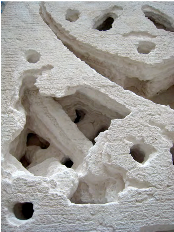
Figure 120 – Photographic detail of printed column section, showing random branching internal geometry and post tensioning conduits.
