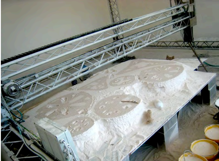
Figure 118 - Commencing sand removal after the 'print' has cured overnight.
