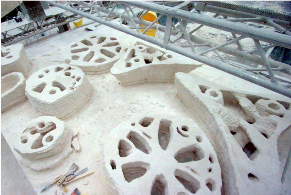
Figure 119 - Parametric column sections on the 'print' bed, revealed after removal of unbonded sand mix. Note object bottom left is cracked, another part further up on the left was also unusable.
