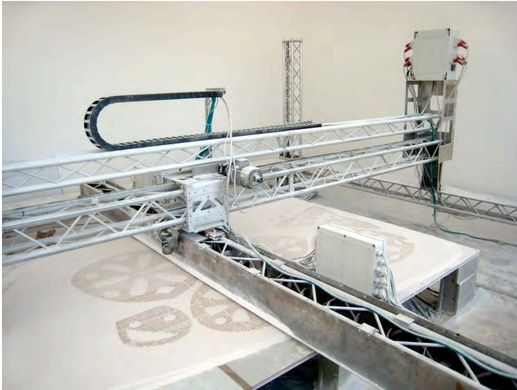
Figure 117 - The D-Shape machine printing the column
