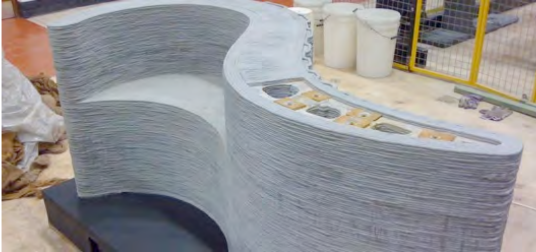
Figure 19 - Concrete Printing Freeform wall test - image source http://www.buildfreeform.com/index.php - Accessed 5th July 2011
