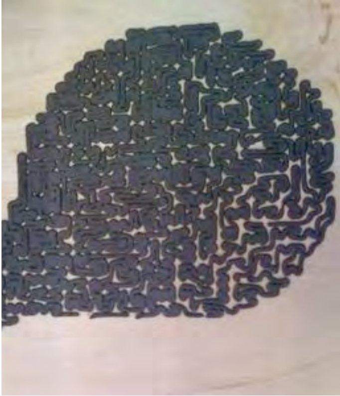
Figure 18 - Example of Concrete Printing test print resolution. Image source http://smarchitecture.blogspot.com/2009/04/freeform-construction-update.html - Image accessed 9th march 2011
