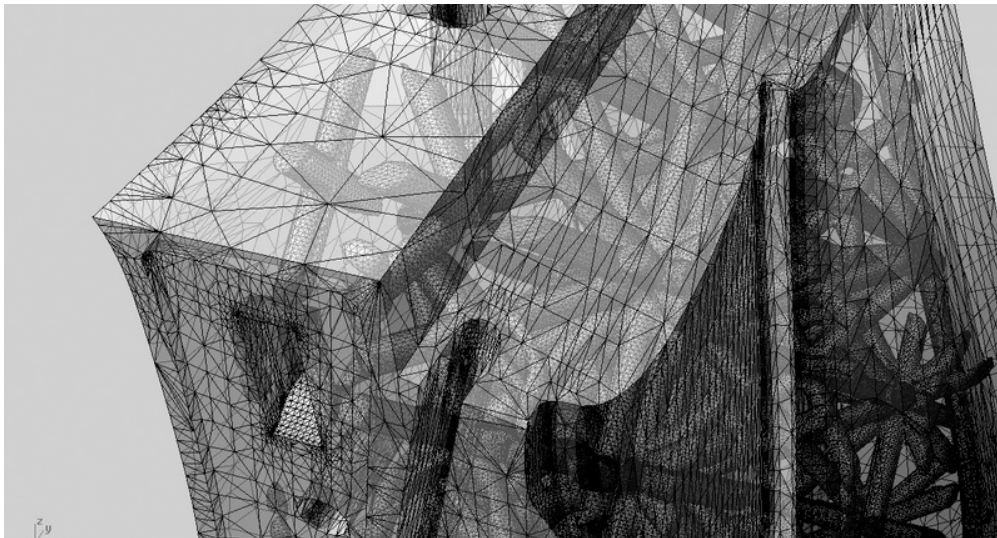
Figure 131 - Ghosted wireframe image of one of the panels before splitting. You can see the internal structure. Image James Gardiner
