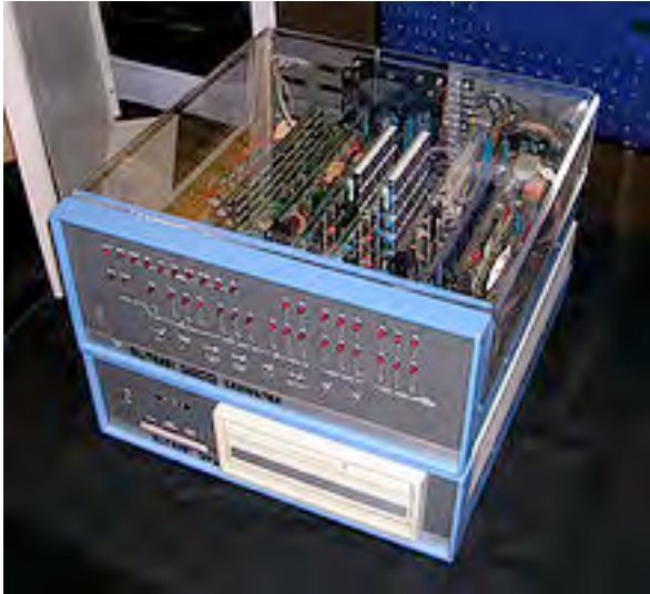
Figure 8 - Altair 8800 the first kit form personal computer. Image source http://en.wikipedia.org/wiki/Altair_8800 - Accessed 8th August 2011
