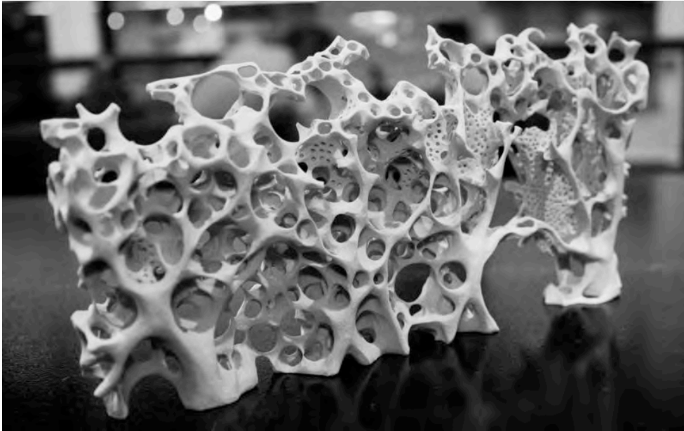
Figure 170 - Design thinking development model. Note the different medium level detail topologies developed: Scalar branching, perforated infill plates.
