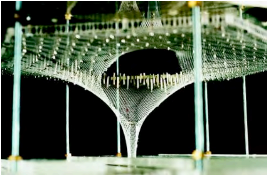
Figure 35 - Experiment by Frei Otto and team for the new high-speed Stuttgart train station - Image source - http://architecturehabitat.blogspot.com/2010/10/final-submission.html Access date 26th August 2011
