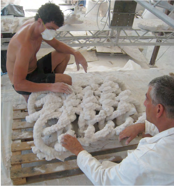
Figure 164 - Interconnected ring test coffee table for Freedom of Creation fabricated by D-Shape™ in 2009. Photo of Enrico Dini and I after removing unconsolidated sand from around the coffee table and lifting it onto the pallet from the print bed. This piece texture looks remarkably like a natural coral structure. Photo James Gardiner
