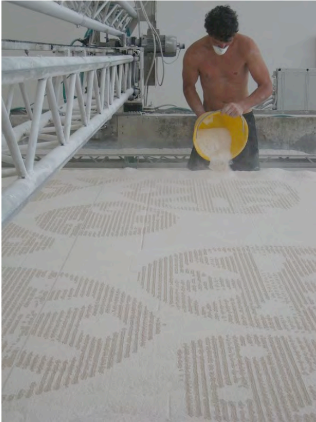
Figure 116 - James Gardiner topping up the back of the sand bed after 1 'print' pass. Note: the gaps left within the 'print' will be filled in by the returning pass.
