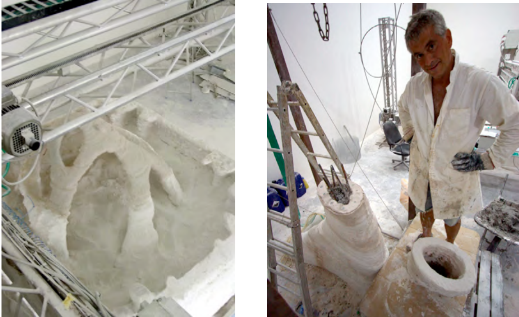
Figure 48 (a) Radiolaria scaled prototype after fabrication, note the external structure around the Radiolaria used to hold unconsolidated sand in place. Image source – D-Shape (b) Testing reinforcement and assembly strategy of D-Shape printed Radiolaria sections at D-Shape factory August 2009. Image source – James Gardiner
