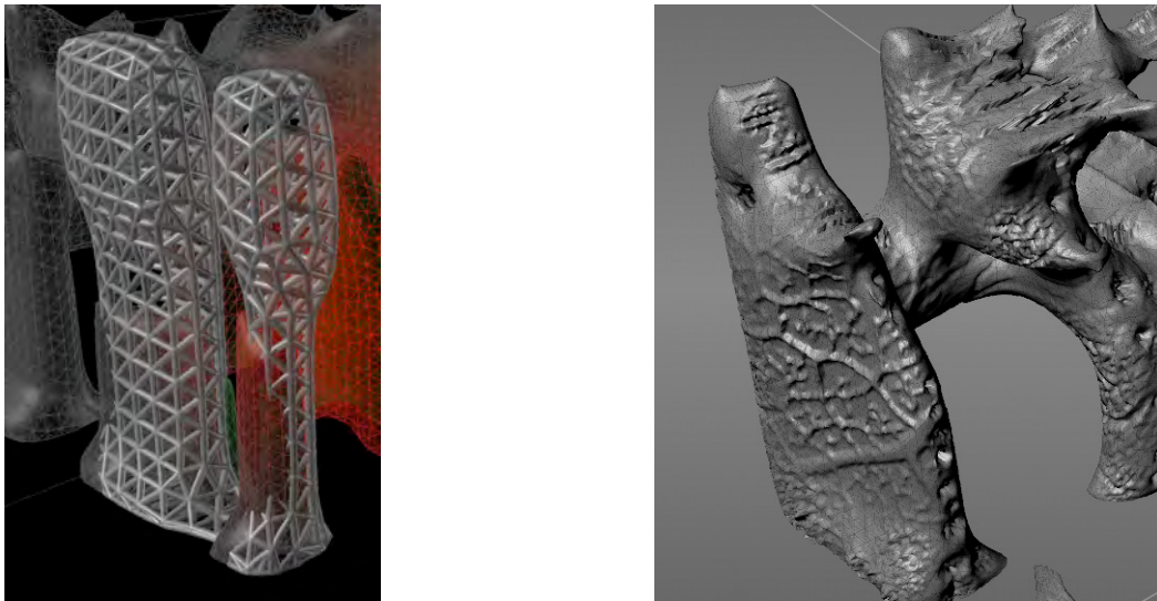
Figure 180 – (a) "piping" the vertices of the envelope mesh with Rhino™. (b) Articulating the inner envelope surface using Mudbox™. Images by James Gardiner
