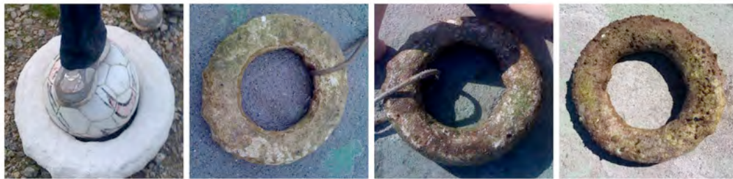
Figure 165 - D-Shape marine testing ring showing flora growth. Photos Nov & Dec 2010, April & August 2011. Images Enrico Dini.
