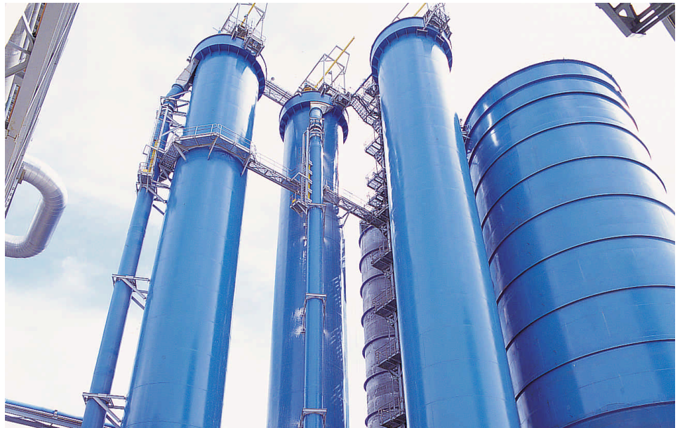
Four-stage ECF bleaching fiberline. Photo by Tom Grow, courtesy of Andritz AG.
