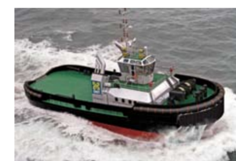
Four 85 tonnes bollard pull 3213 ASD tugs were ordered in May 2007.
