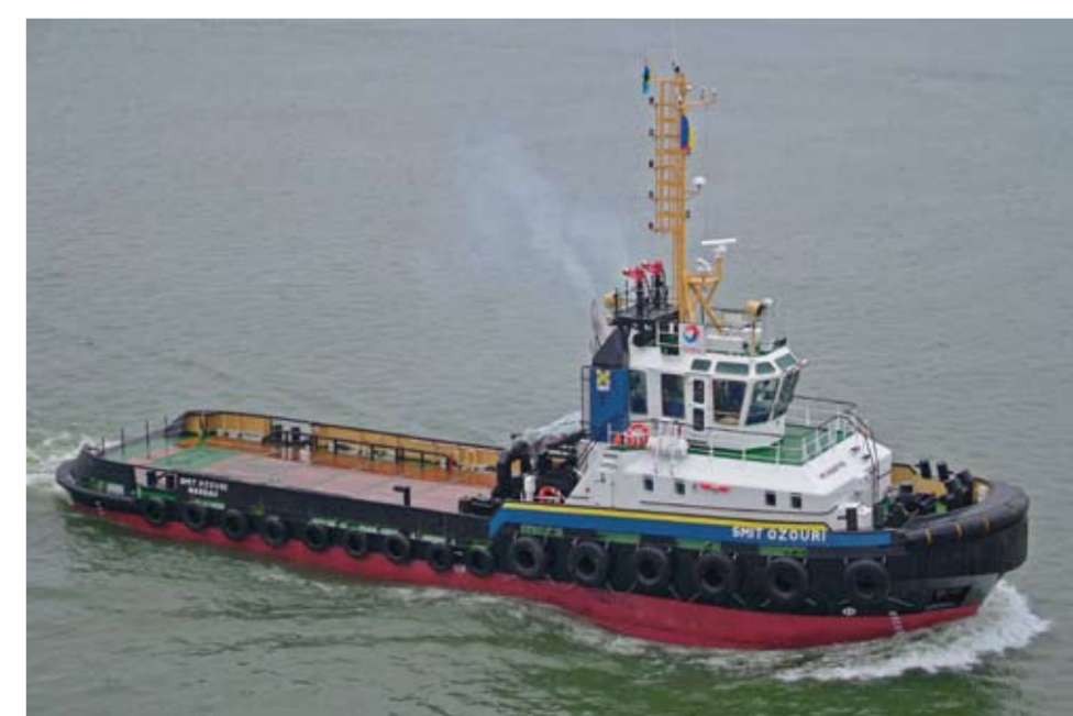
3509 stan tug 'Smit Ozouri' was delivered at the very end of 2006 and is now deployed in Port Gentil, Gabon.
