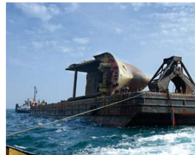
Following the stern, the bow of the 'Michelle' was lifted and removed.
