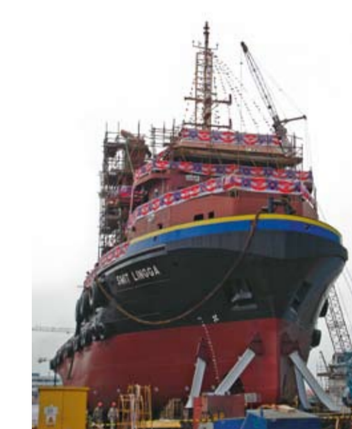
One of the new AHTS vessels under construction at the Keppel Singmarine yard in Singapore.
