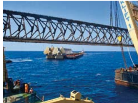
Sheerlegs 'Taklift 1' during the recovery of the remaining legs of jack-up rig 'High Island 3'.
