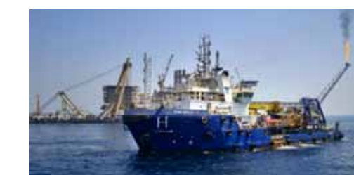
DP2 DSV 'Team Muscat' was mobilised with SMIT Subsea's SAT3 system to recover the legs of rig 'Noble David Tinsley'.
