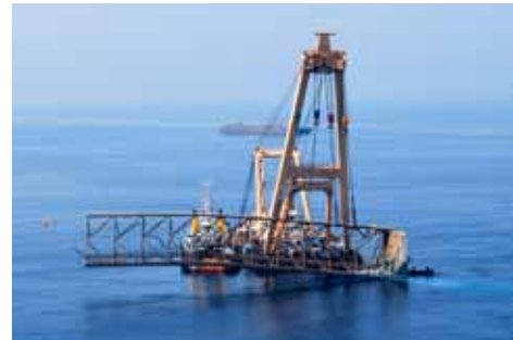
Sheerlegs 'Smit Cyclone' with one of the legs of the rig 'Noble David Tinsley'.
