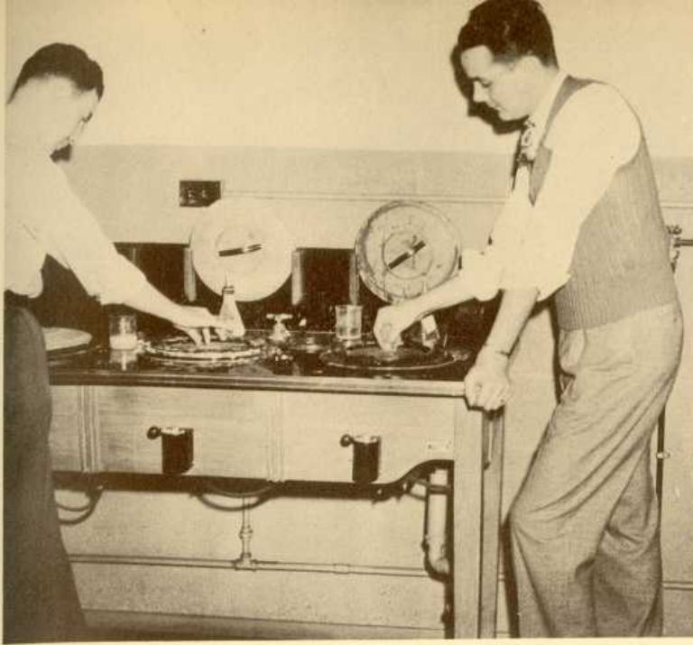
THEY APPEAR confident that their work will be a success while working in the Towne School lab. These Metallurgical Engineering Students are polishing brass specimens.
