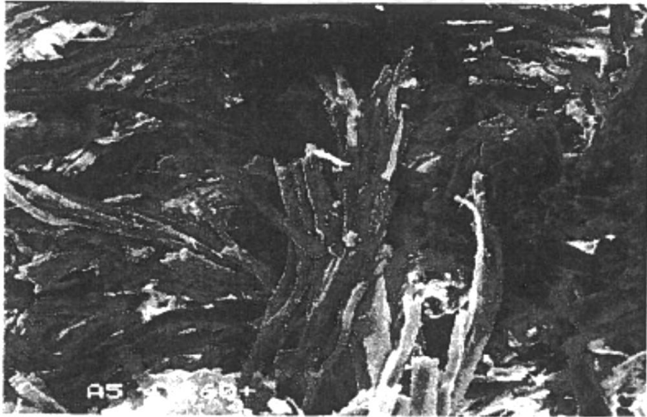
Fig. 1. Photomicrograph of gold coated leather sample n. 4, under the SEM, magnification 260x.
