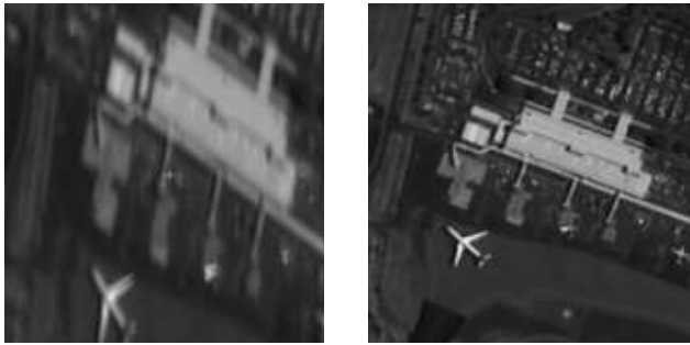
Figure 5.0 Cartosat-2 Image acquired in 0.4m GSD (a) RAW (0.4m x 0.8m) (b) Rad sum: PSF corrected 0.8m x 0.8m
