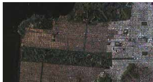
Figure-4: Polarimetric combination showing clear distinct between different bounces.
