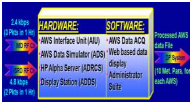
Figure-3 AWS Data Reception System Configuration
