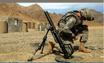
Man-portable, lightweight, smoothbore muzzle-loaded mortar with high angle of fire and improved rate of fire capability. Fires the full family of 60mm mortar ammunition; High Explosive (HE), Smoke, Illumination (Visible and Infrared) and Practice.
