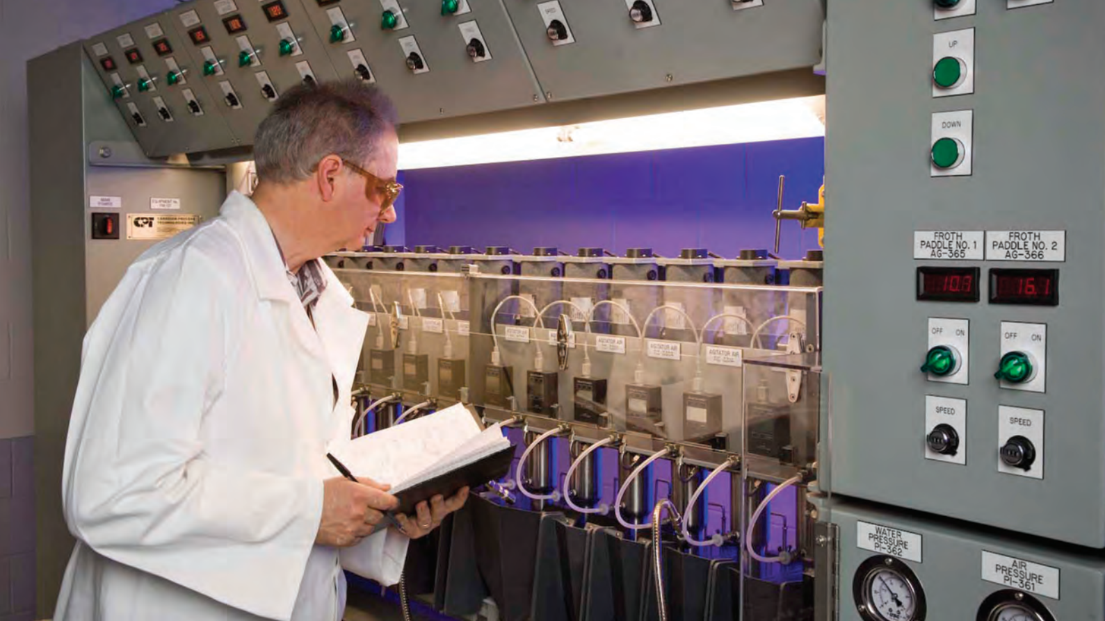
Mr Keith Quast with The Wark's Mini Pilot Flotation Plant.
