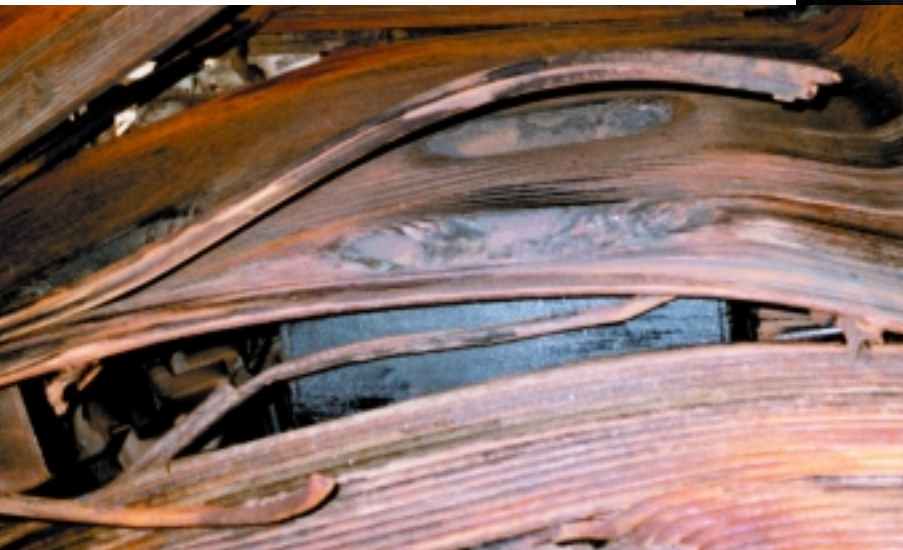
Above: Tube failure due to local overheating.
