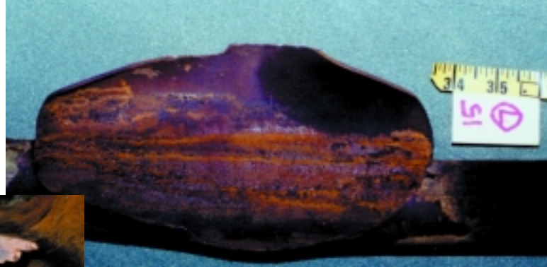
Above: Tube failure due to local overheating.
