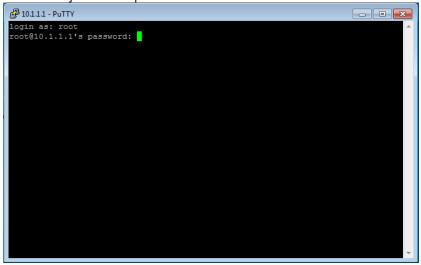
8. Type "runStickCal.sh" and hit enter. (Note: type "runS" and hit "Tab" to complete the command).
