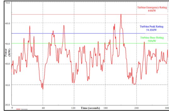
Figure 8: Generator Supplying Demand of Entire System
