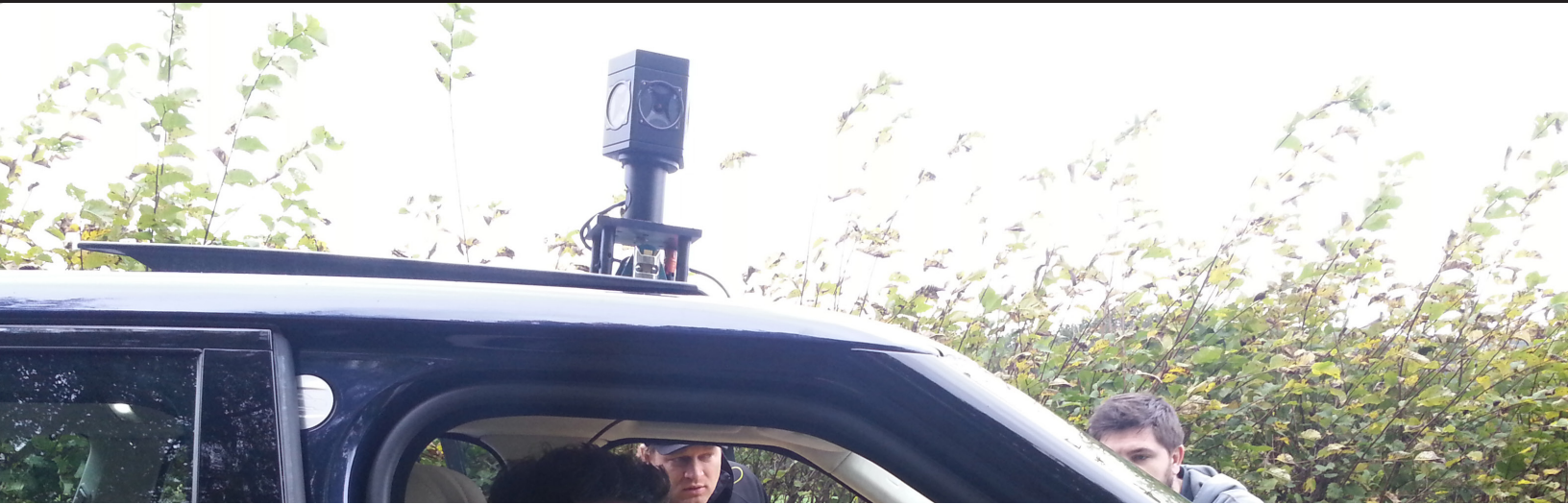
Hex camera mounted on a vehicle utilizing one of Immersive Media's optional vehicle mounting kits.
