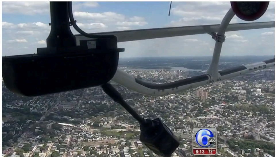
Hex camera pole mounted on retractable permanent helicopter mount . (Courtesy of WPVI Philadelphia)
