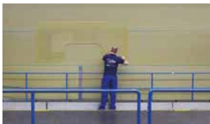
Operator working on Glare® fuselage panel for the Airbus A380 at Fokker in Papendrecht
