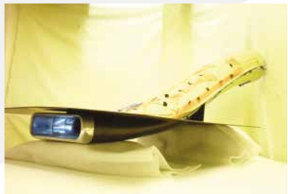
GKN Aerospace's quieter, rugged lightning and ice protected air intake developed through the SIPAL programme
