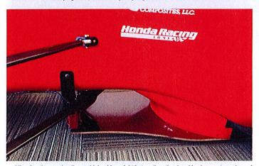
... Likewise the wooden floor, which adds weight but on the other hand is cheaper to make and to replace, so while it may seem a little agricultural for a modern racecar it should be effective
