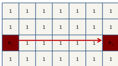
Figure 6. A direct pipeline between two points on the baseline uniform cost surface
