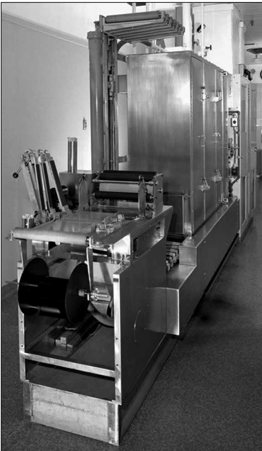
Figure 18: Dalton Duplicate Film Processor. Photo from archives of Bridgehead's Special Programs unit.
