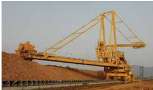
Bauxite stacker reclaimer, Vedanta Limited - Lanjigarh
