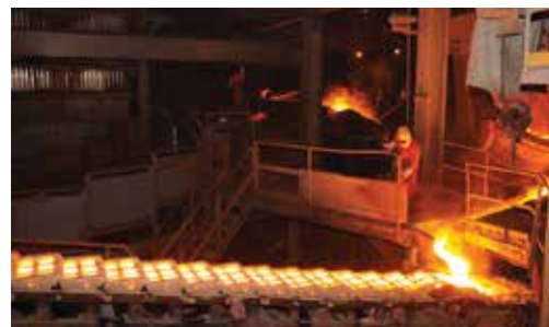
Hot Metal poured into Pig Casting Machine at the Pig Iron Plant: Goa
