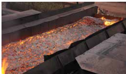
Hot Coke being pushed in the Coke Machine at the Met Coke Plant: Goa
