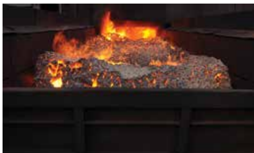
Hot Coke being pushed into the Coke Machine for Quenching; Met Coke Plant at Goa
