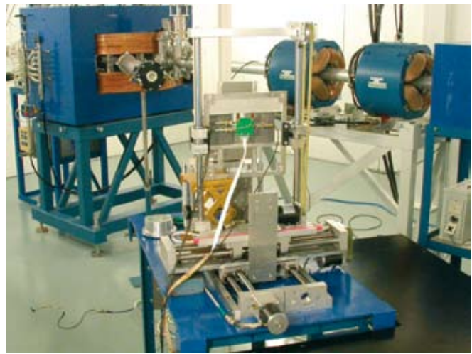
Radiation hardness tests at JYFL of T0 and V0 detectors for ALICE experiment.
