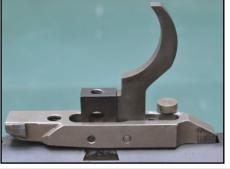
The CAM most be one of the most simple and substantial trigger mechanisms I have ever worked with and as a result component and combat failure rate must be absolutely minimal. Similar to the Mauser system the whole assembly is held in place by two pins and to remove the bolt the user must pull the bolt to the rear and at the same time fully depress the trigger. I polished the sear and cocking piece bearing surfaces and by adjust the trigger screw reduced the trigger pressure to 3.9lbs.
