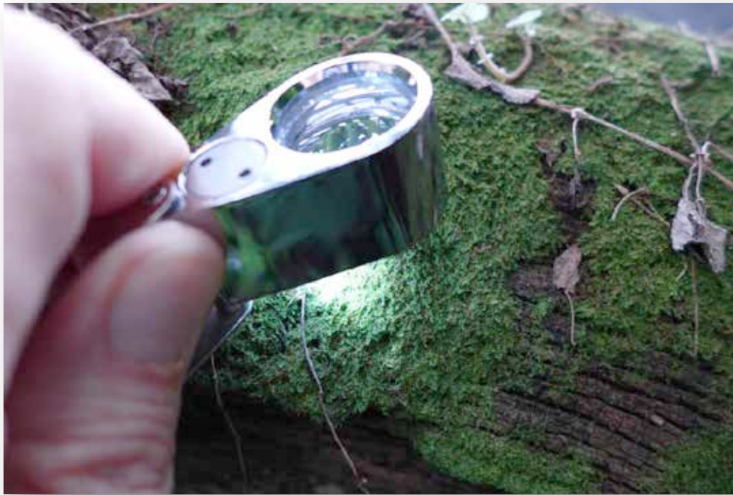
Figure 3 Despite its size, this hand lens with built-in LED lamp is very useful in dark forests. The lens quality is mediocre.
