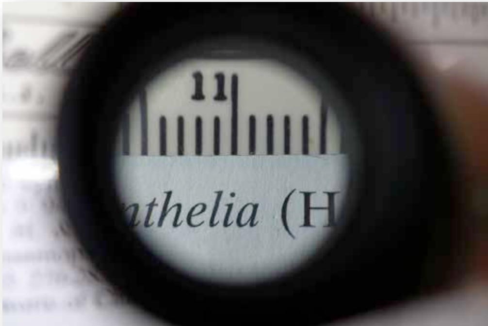
Figure 2 The view through the Iwamoto Achromatic 20x hand lens show remarkably little optical aberrations. The view is crisp and clear.
