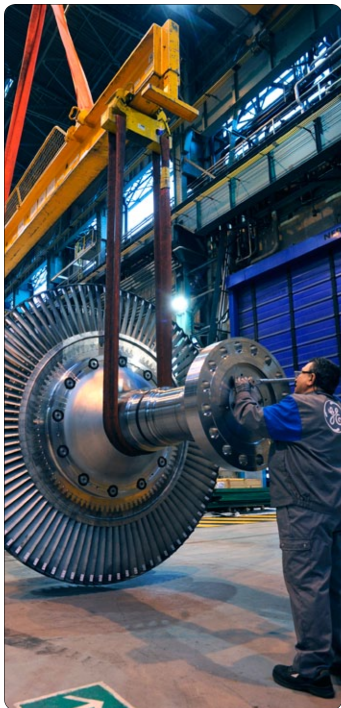
A General Electric employee assembles a component for a gas turbine at the company's factory in Belfort, France
