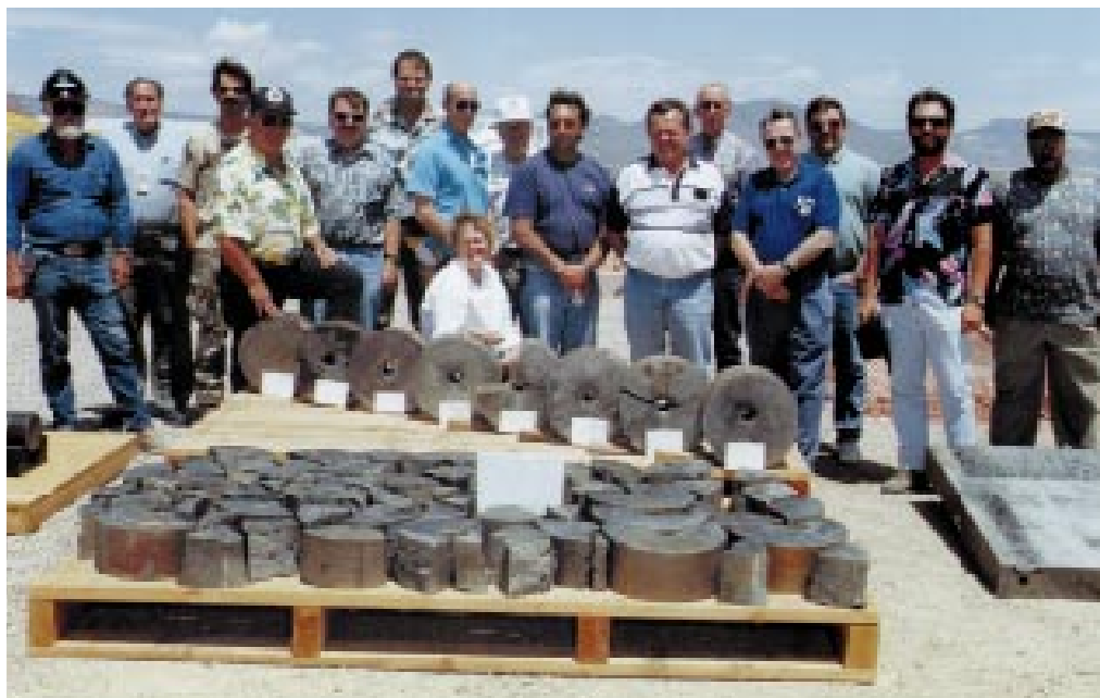
Figure 1. Testing personnel stand behind perforated blocks of armor steel after the early 1997 shaped-charge demonstration at the Nevada Test Site.
