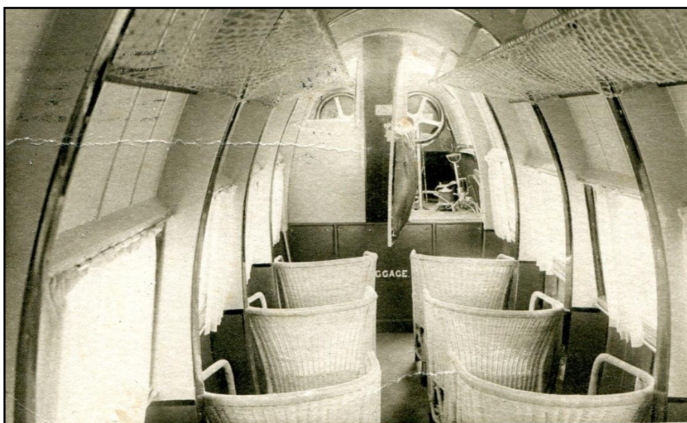
The interior of Imperial Airways aircraft, note the cane seats for passengers, not I would suggest very comfortable for long air journeys.
