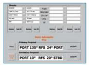
The large flat panel touch sensitive display on the CU gives easy access to all relevant information. For manual operation the tube or tubes to fire is simply pressed and the selection acknowledged by a press on the separate hardwired fire key on the Control Unit front panel. Firing can only be executed if the Control Unit safety key switch is in armed position.
