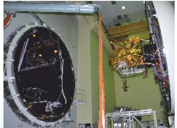
IRNSS-1F being loaded into thermo-vacuum chamber
