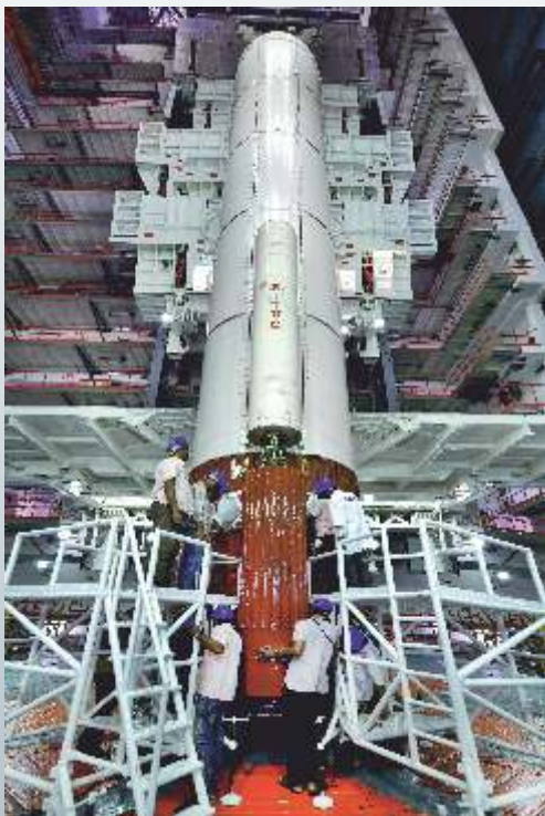
Assembly of PSLV-C32 First stage in progress
