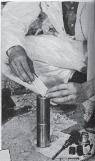
Small test rocket is loaded into firing stand, upper left, to trace its characteristic path. Above, putting powder charge in rocket. Diagram shows man's altitude records and his hopes for the rocket
