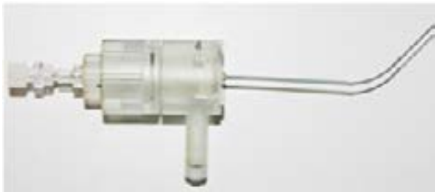
Innovative MR compatible applicator for percutaneous intradiscal thermotherapy
