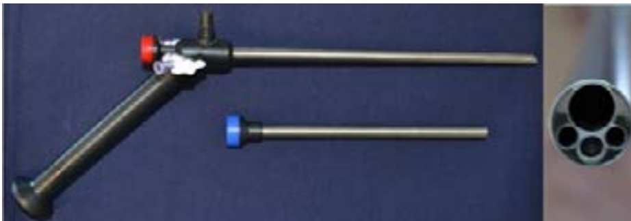
PEEK prototype of the multifunctional endoscopic device
