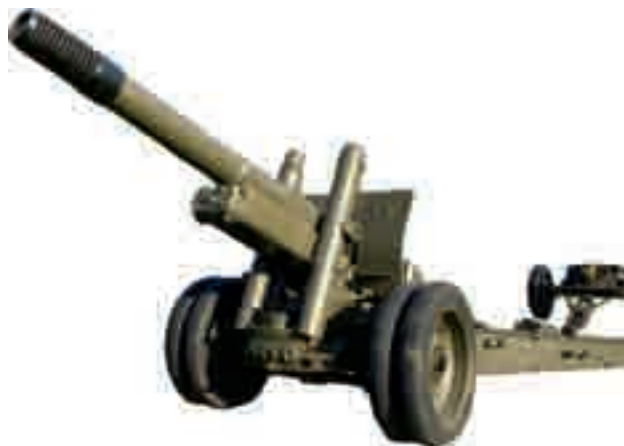
Tunul-obuzier ML-20, calibrul 152 mm, model 1931/37
