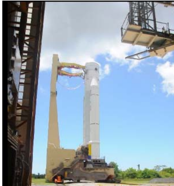
Kourou: transfer of the launcher from the Launcher Integration Building (BIL) to the Final Assembly Building (BAF)
