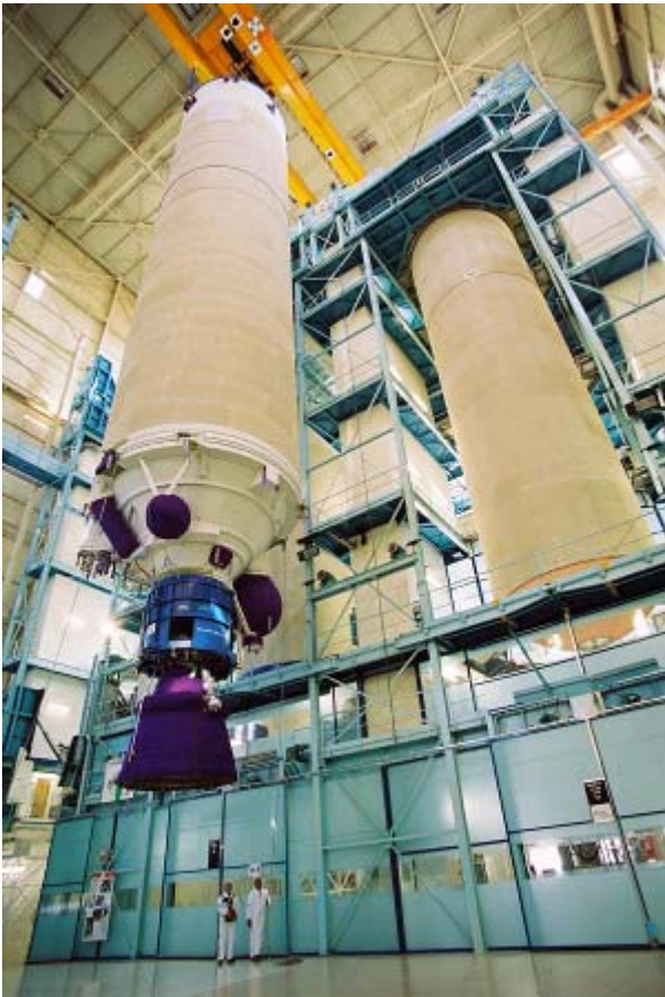
The Ariane 5 main cryogenic stage (EPC) in the integration dock at Les Mureaux, France, in course of preparation for tilt and containerization
