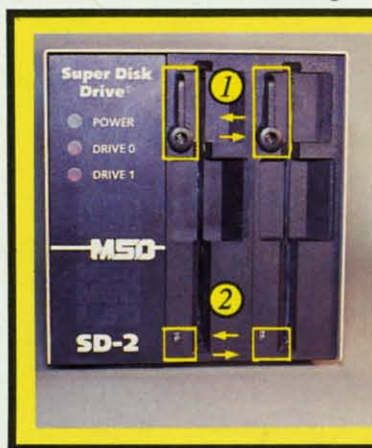
PHOTO 1: Front panel of MSD Dual Disk Drive. Disks are inserted vertically and secured by twisting and locking levers a quarter turn. READER SERVICE NO. 4
