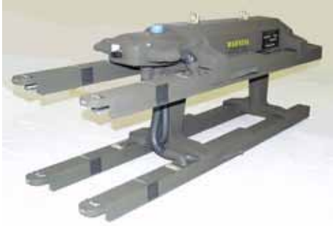
The M299 Smart Launcher is capable of firing all HELLFIRE missile variants.
