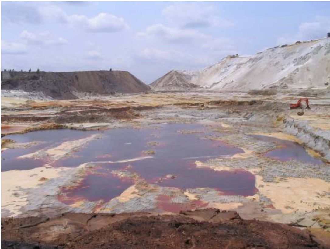
Figure 6.1. AMD formed owing to interaction between water and mine residues on the surface, exposed in a surface tailings reclamation operation in the Western Basin. Note that this site drains into open pit operations that are directly connected to the mine void
