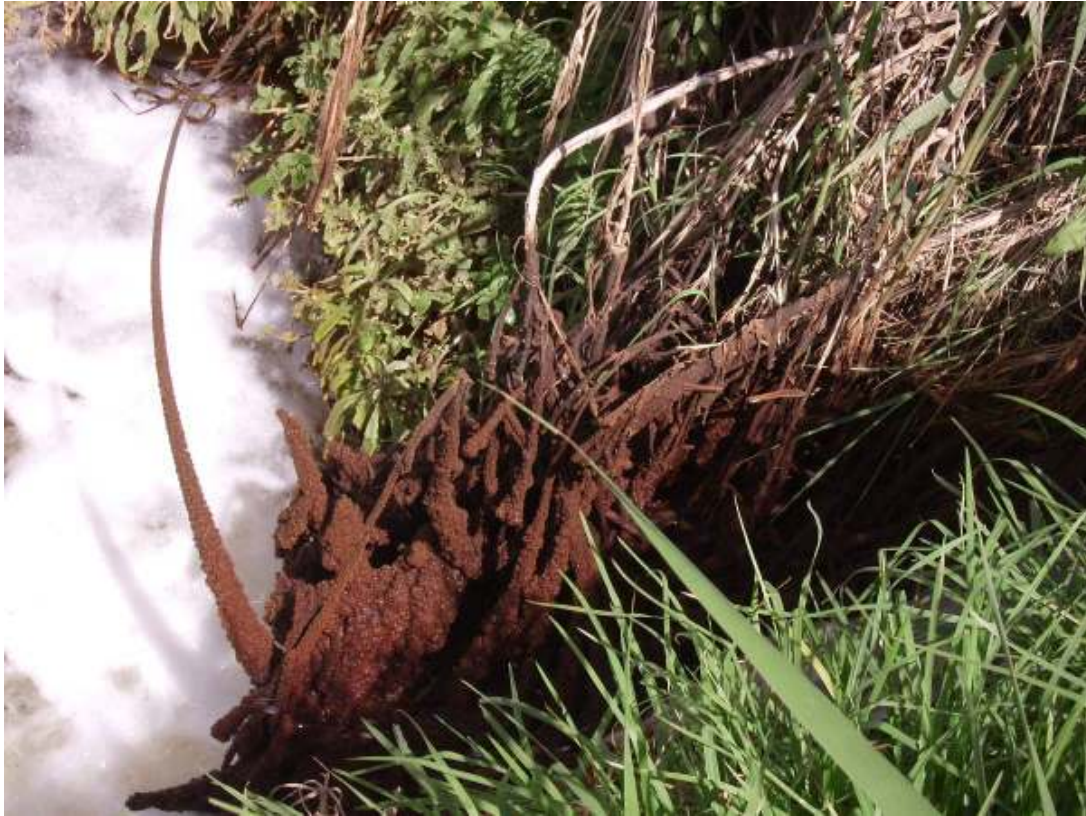
Figure 6.5. Salt crusts precipitating on vegetation downstream of the decant from the Western Basin
