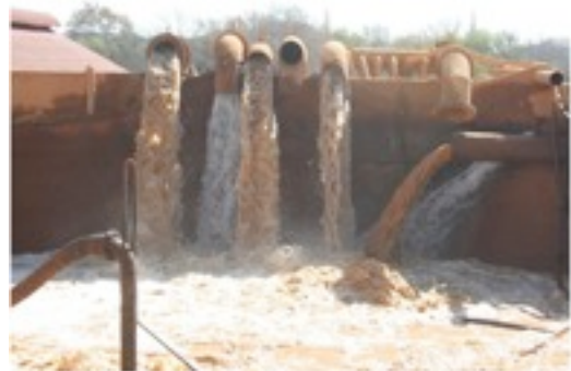
Mine water being pumped from the Eastern Basin
