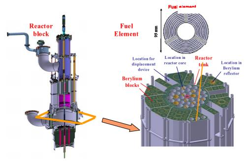
Fig 2. View of the reactor core with experimental locations
